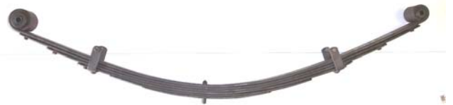
< FRAME END (LARGE BUSHING) – PHOTO 4 – SHACKLE END >
